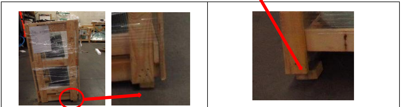
Removal of the cover boards (of the cover)
